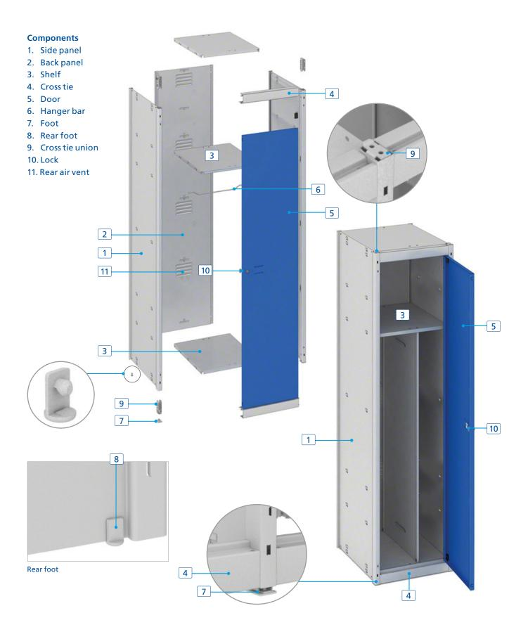
4 Metal lockers mecalux.com.tr
